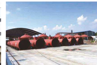
河南太康建材公司 6条31米蒸压釜和8吨冷凝燃气蒸汽锅炉 6 sets 31m autoclaves and 8T condensing gas steam boiler for Henan building materials company
