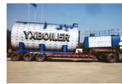
江苏酒厂 20吨燃气冷凝锅炉 20t/h gas condensing boiler in Jiangsu brewery
