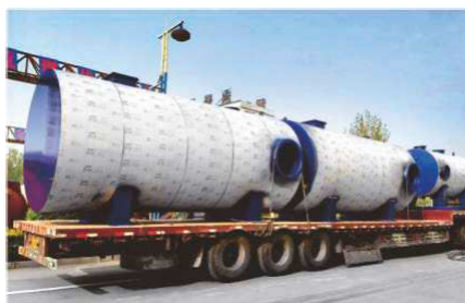
新疆 3台120万大卡热风炉用于烘干棉花 3sets 1,200,000kcal hot air furnaces for Xinjiang cotton drying
